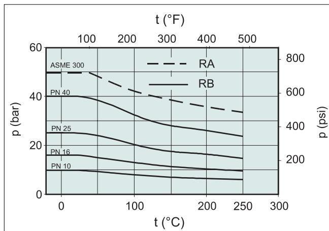
Note that max. throttling pressures are mechanical maximum differential pressures at ambient temperature.
